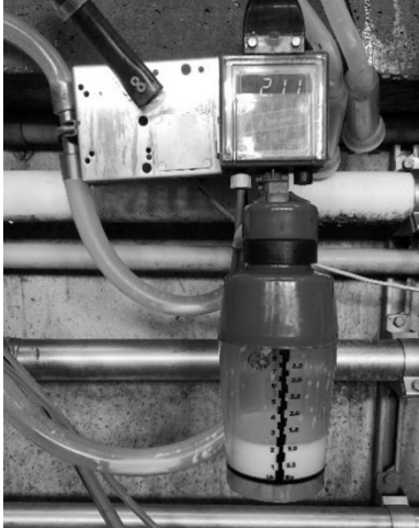
Figure 3: This is one of our DeLaval samplers. The sampler connects directly to the milk meter.
