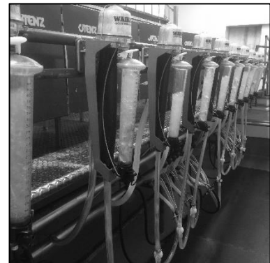
Finished metering, meters washing with the CIP system after milking
